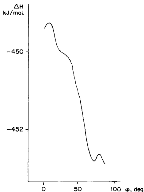
Fig. 1. The potential energy curve relating to internal rotation of the \text{CF}_3 group about the \text{C}_1 -S bond for compound 1 (for notes see Table 1).
